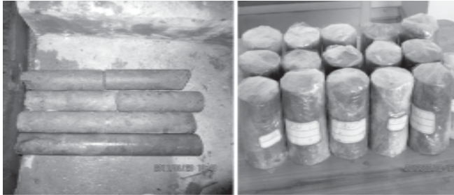
(a) Taking rock samples on site (b) Processed rock specimens Fig.1 Rock specimens
