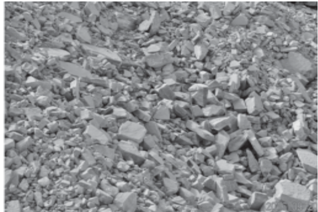
Fig.3 Image of the blast fragmentation obtained
