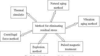
Fig.3 Residual stress relief methods
