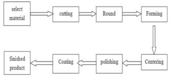
Fig.1 Traditional aspheric mirror processing flow
