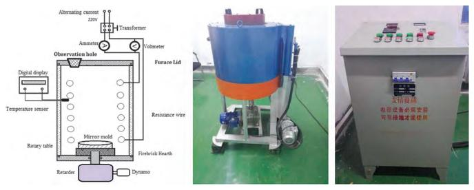
Fig.2 Centrifugal casting system and control cabinet
