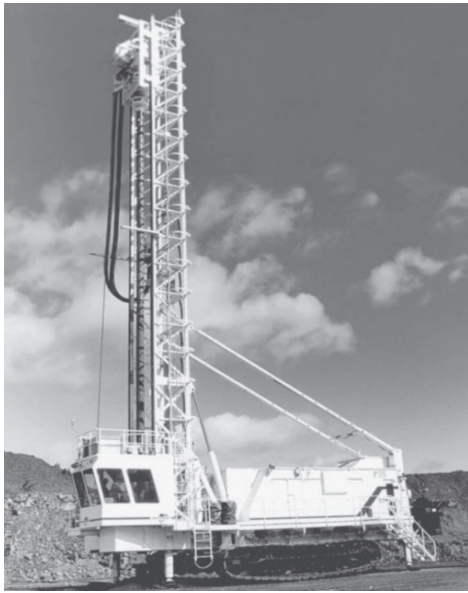
Fig.2 A blasthole drill rig
