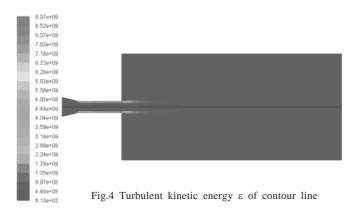
dissipation rate of turbulent kinetic energy distributes in the following locations: convergence angle, inner wall of the cylinder and nozzle outlet.
