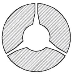
Fig.7 Profile of drill pipe
