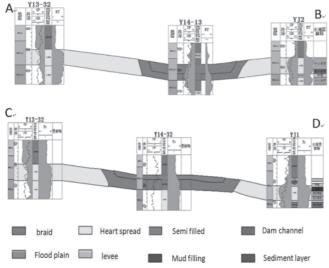
Fig.6 Well section of channel sand with mud semi-filling in Y3H12 well area
