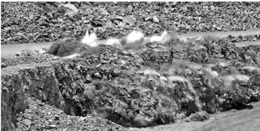
Fig.7 No stemming ejection, proper face movement, no fly rock
