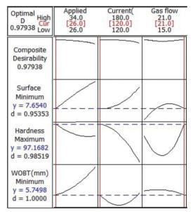
Fig.15: Multi objective optimization of hardness, WOBT and SR
