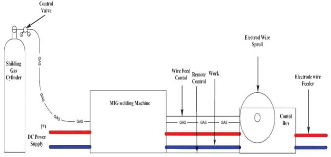
Fig.1 Schematic diagram of MIG welding machine
