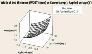
Fig.9 Effects of applied voltage and current on WOBT
