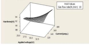
Fig.6 Effects of applied voltage and current on hardness
