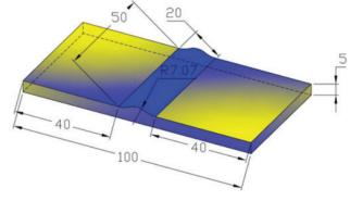
Fig.5 3D drafting model of welding spot
