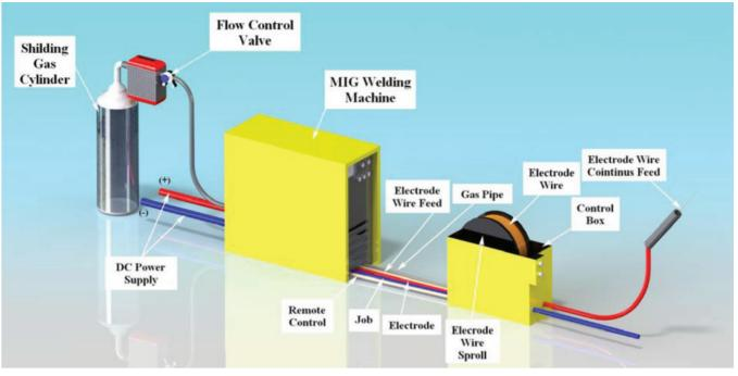
Fig.2 3D model of MIG welding machine
