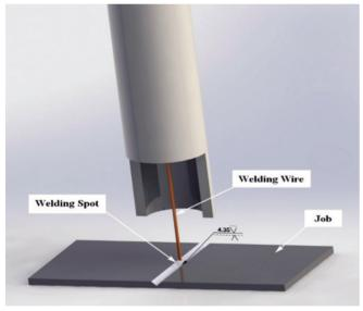
Fig.3 3D model of welding spot with welding wire
