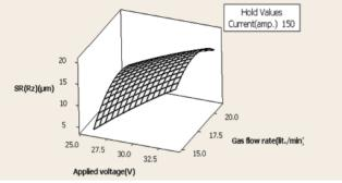
Fig.11 Effects of applied voltage and gas flow rate on SR
