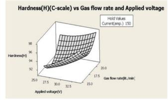
Fig.7 Effects of applied voltage and gas flow rate on hardness
