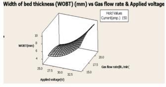
Fig.8 Effects of applied voltage and gas flow rate on WOBT
