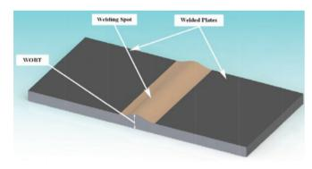
Fig.4 3D solid model of welding spot
