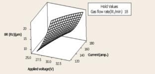
Fig.10 Effects of applied voltage and current on SR
