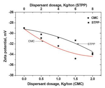
Fig.1: Zeta potential of the coal as a function of CMC and STPP as a dispersant
