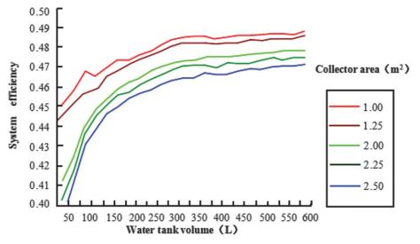
Fig.7: Influence of different heat collecting area and corresponding water tank volume on solar energy guarantee rate
