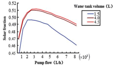
Fig.10: Influence of different water tank capacity and corresponding water pump flow rate on solar energy guarantee rate
