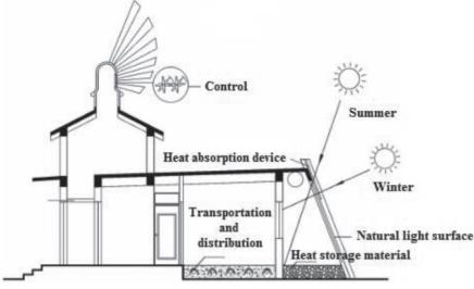
Fig.1: Sketch of the five elements of passive solar energy utilization
