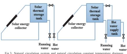
Fig.3: Natural circulation system and natural circulation constant temperature drainage system
