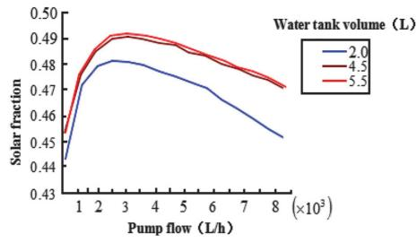
Fig.11: Influence of pump volume and volume of water tank on solar energy efficiency under  $30m^2$  heat collecting area
