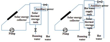
Fig.4: Direct forced circulation system (left is single tank, right is double tank)
