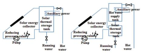
Fig.5: Indirect forced circulation system (left is single tank, right is double tank)
