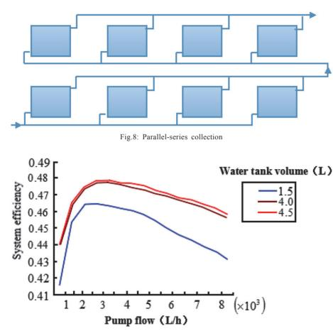
Fig.9: Influence of different water tank capacity and corresponding pump flow rate on system efficiency
