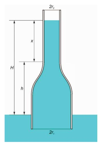
Fig.3 The capillary tube with an uneven cross-sectional radius
