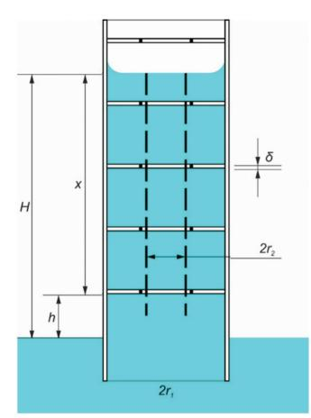
Fig.4 The capillary with perforation holes
