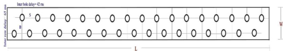
Fig.4 The layout of blast round with two rows
