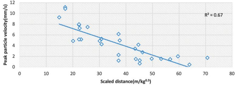
Fig.8 PPV vs SD graph for 26-50 number of holes
