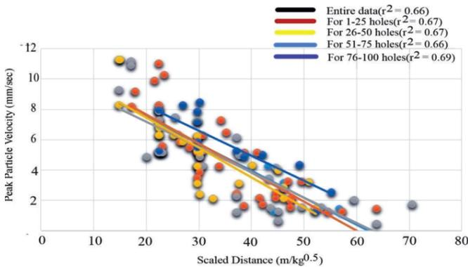
Fig.11 PPV-SD graph for comparison of data sets of grouped holes and entire data
