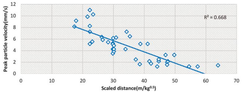
Fig.7 PPV vs SD graph for upto 25 number of holes
