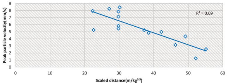
Fig.10 PPV vs SD graph for 76-100 number of holes
