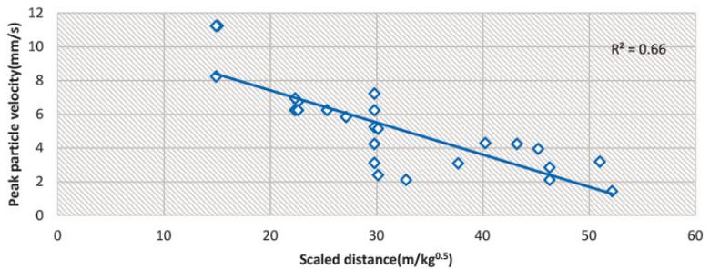
Fig.9 PPV vs SD graph for 51-75 number of holes
