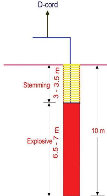
Fig.5 Representative charged blast hole section (not to scale)
