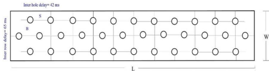
Fig.3 The layout of blast round with three rows
