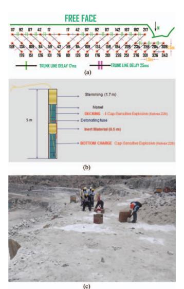
Fig.4 (a) Initiation pattern (b) Modified charging geometry with 'decking' (c) Charging of holes in the site
