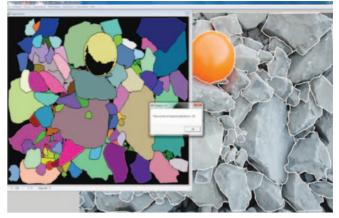
Fig.1 Fragmentation analysis using image analysis software
