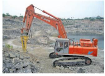
Fig.8 Rock breaker working with blasted muckpile
