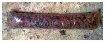
Fig.7 Cartridged packing of crushed angular stones used for 'decking'
