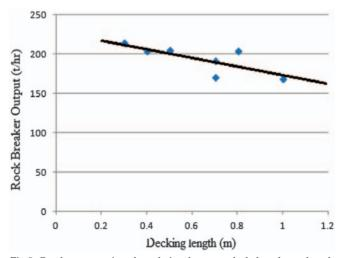
Fig.9 Graph representing the relation between deck lengths and rock breaker performance
