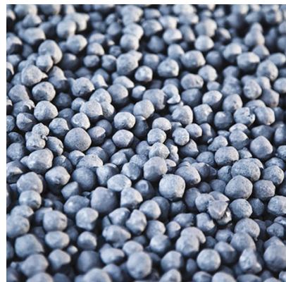
LKAB's iron ore pellets are made from magnetite and have high iron content, around 67 per cent.
