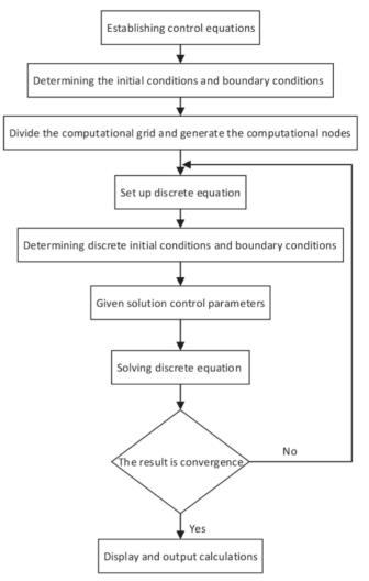
Fig.1 Work flow diagram of CFD
