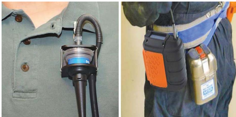
Fig.3: Procedure for wearing the Airtec instrument for collecting DPM
