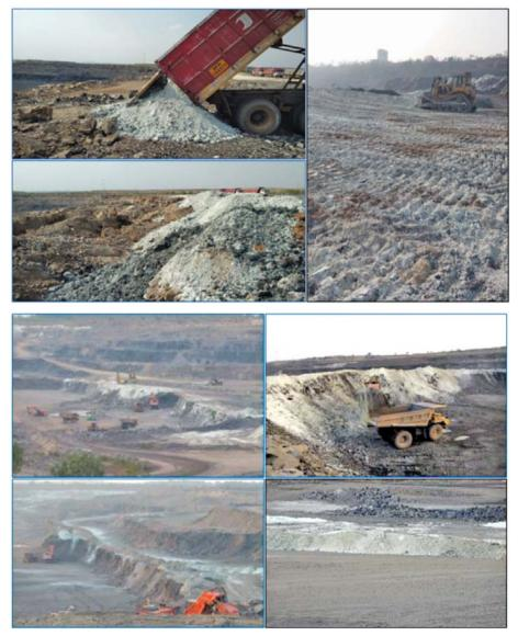
i.e. transfer points chutes getting jam due high moisture and it is tedious job to clean, hampers the crusher/conveying system. The process started by unloading lime sludge near crusher hopper feeding started by wheel loader with ROM limestone feeding as there is no suitable arrangement to feed
