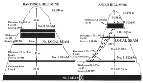
Fig.2: Section showing surface and seam profile (DGMS, 2010)
