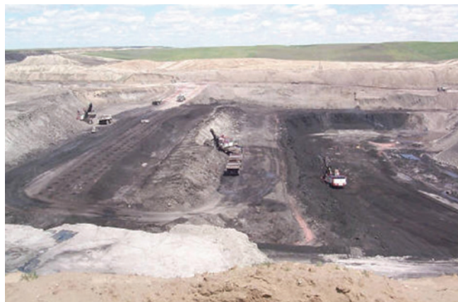
Drive-by layout, Wyoming Coal – trucks positioned parallel to digging face, with no back-up drive required – operation became a “Rock Factory”, critical to survive in a razor-sharp margin business
