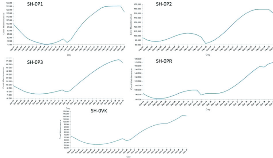
Fig.7: Total optimised maintenance cost of mining shovels
