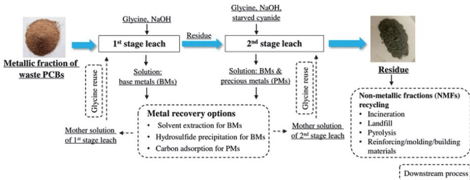
The likely method (not verified) (Text and figure reference: Elsayed A. Oraby, Huan Li and Jacobus J. EksteenWaste and Biomass Valorization volume 11, pages 3897-3909 (2020)" An alkaline glycine-based leach process of base and precious metals from powdered waste printed circuit boards"
