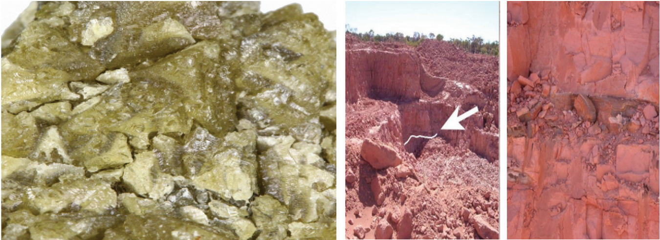
Fig.2: Presence of 'floaters' in the soft rock matrix
