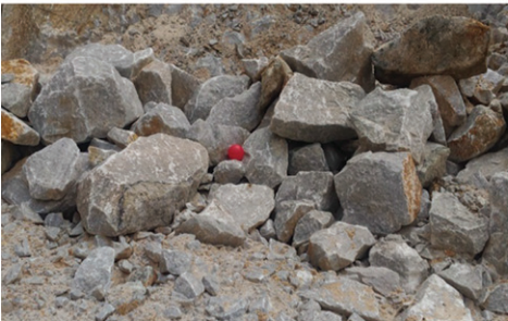
Fig.7: Improved fragmentation of muckpile using V initiation system blast design
