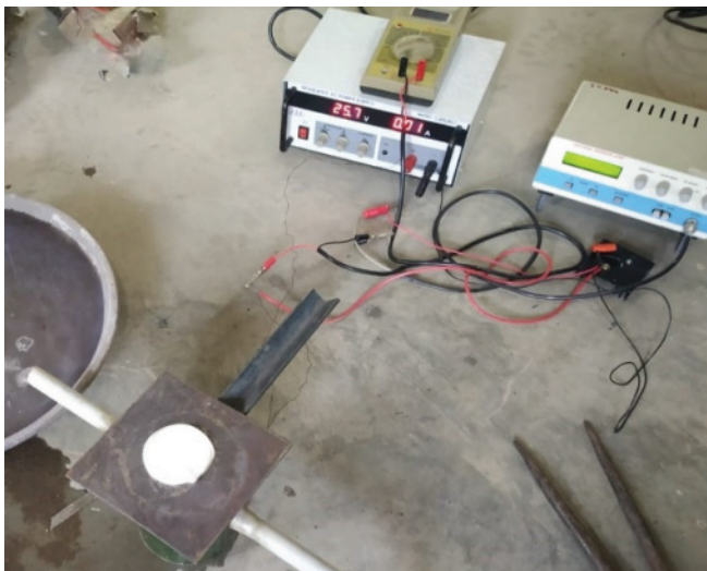
Fig.1: Ultrasonic module with die during casting
