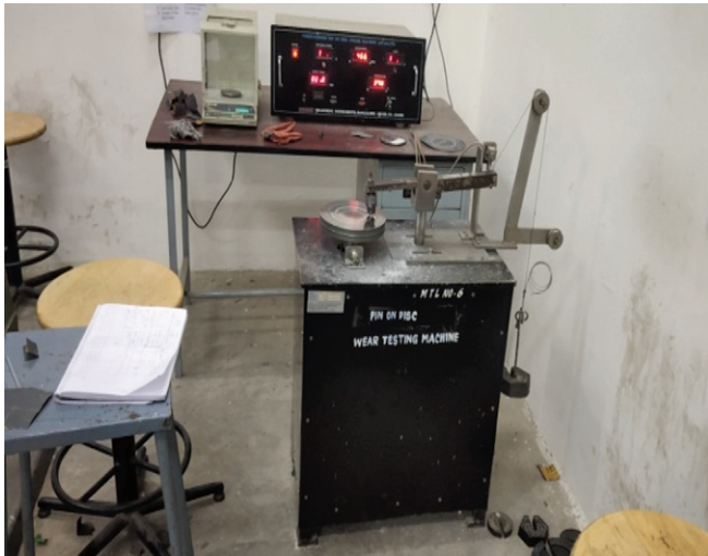
Fig.4: Pin on disk tribometer
