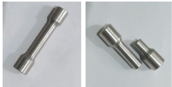
Fig.2(a): Tensile test specimen (before test) (b): After tensile test
