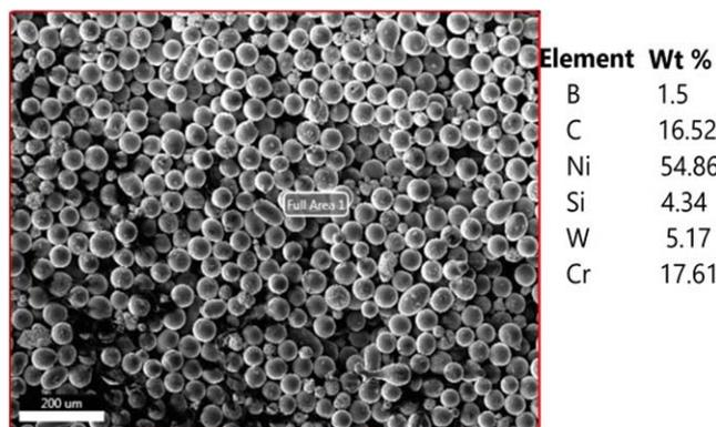
Fig.1: SEM with EDAX of alloy powder
