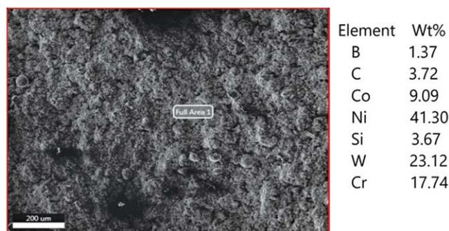
Fig.2: SEM with EDAX of (30%WC-CO+NiCrBSi 70%) coated Superco-605
