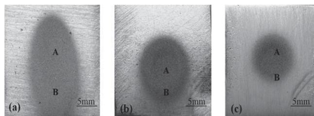
Fig.3: Images of erosion scar on bare Superco-605 at three different impingement angles (a)  $30^\circ$  (b)  $60^\circ$  and (c)  $90^\circ$
