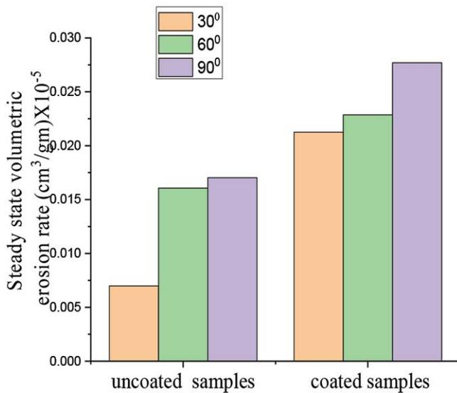
Fig.10 comparison of plots of steady state volumetric erosion rate of coated and bare samples
