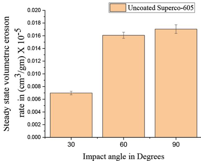
Fig.5: plot of steady state volumetric erosion rate for different impact angle
