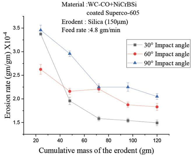
Fig.7: Plot of the erosion rate vs accruing mass of the erodent
