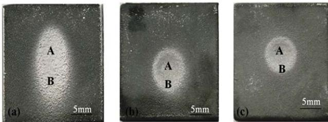
Fig.6: Erosion scars developed on (30% WC-CO+NiCrBSi 70%) coated Superco-605 sample at three different angle of impingement (a) 30° (b) 60°, and (c) 90°
