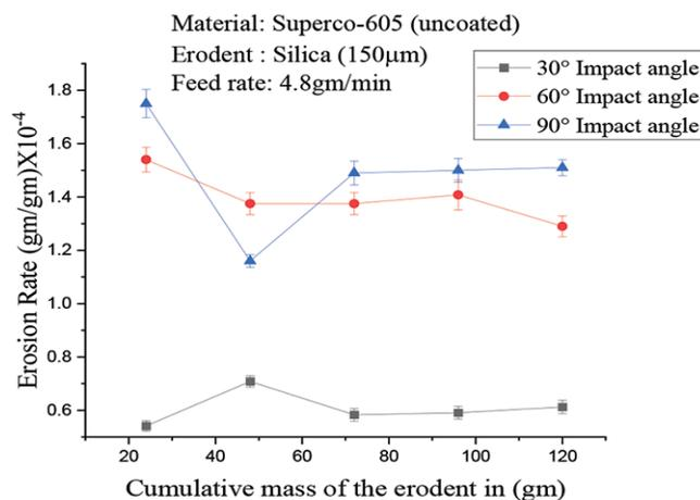
Fig.4: Plot of the erosion rate v/s accruing mass of the erodent
