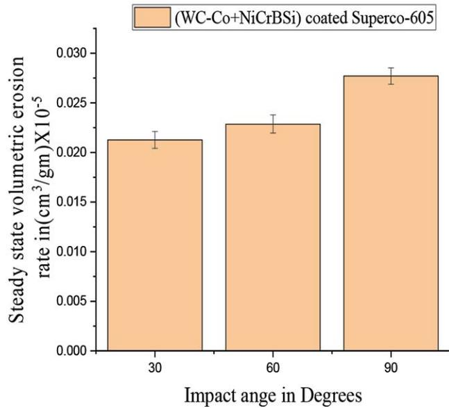
Fig.8: steady state volumetric erosion rate for different impact angles
