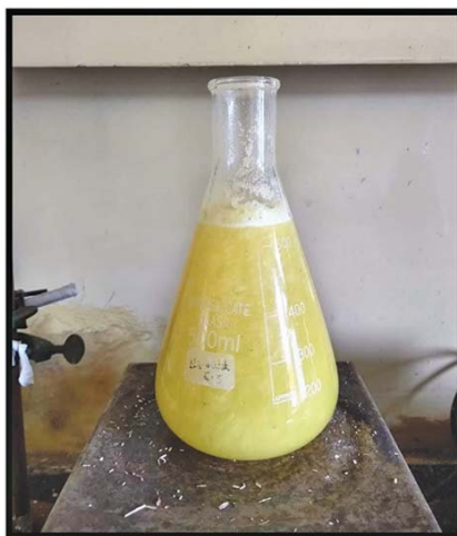
Fig.5: Acetylation using buffer solution
