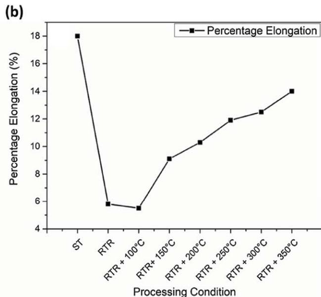
Fig.3. Variation of strength and elongation to failure of Al-Li 8090 alloy for different processed conditions (a) UTS and YS variation, (b) percentage elongation variation
