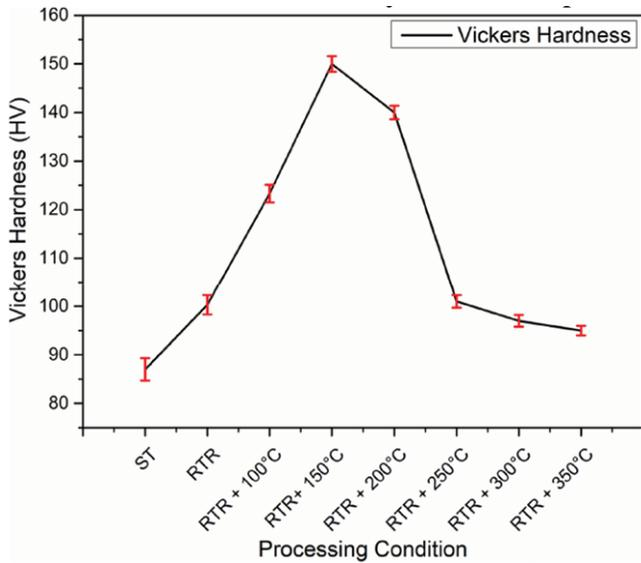
Fig.2: Variation of hardness of Al-Li 8090 alloy for different processed conditions
