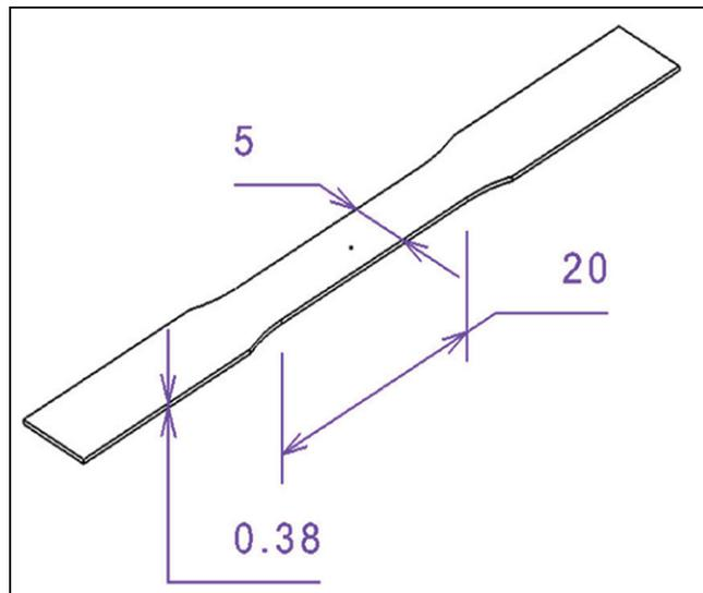
Fig.1. Specification of tensile specimen in mm
