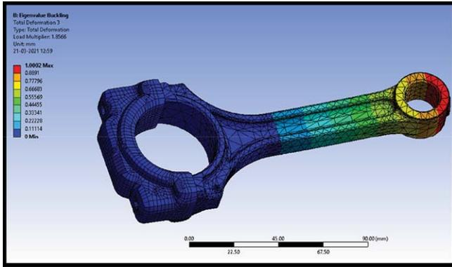
Fig.6: Buckling load factor plot and front view of buckling load factor plot ti alloy
