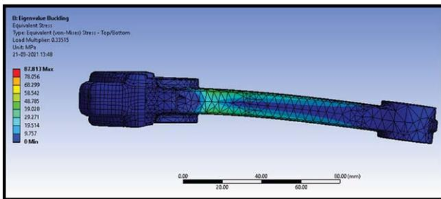
Fig.7: Von-mises stress plot and zoomed in view of maximum stress plot mg alloy (side view)
