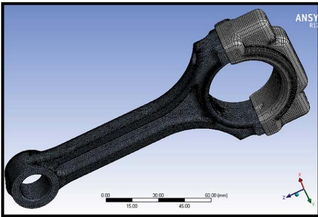
Fig.2: Finite mesh of connecting Rod
