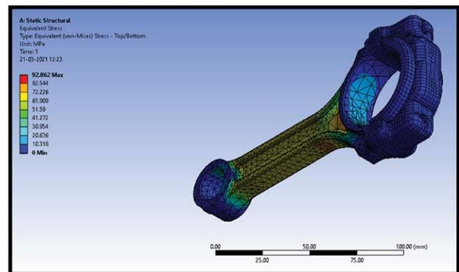
Fig.5: Static Structural representing Von Mises stress for Ti Alloy at different orientations at side view
