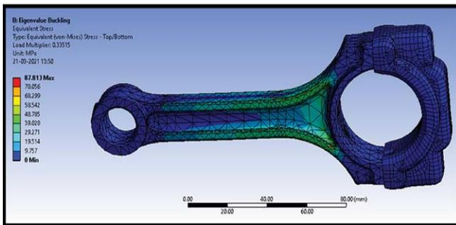
Fig.8: Von-Mises stress plot and zoomed in view of maximum stress plot mg alloy (front view)
