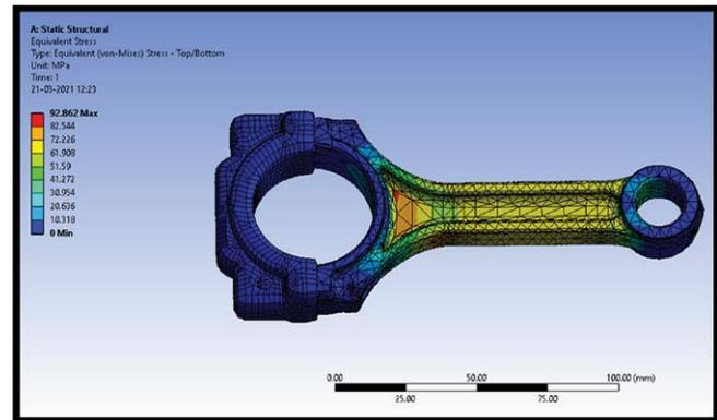
Fig.4: Static structural representing Von Mises stress for Ti Alloy at different orientations front view
