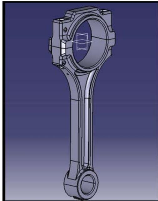
Fig.1: 3D model view of diesel generator connecting rod
