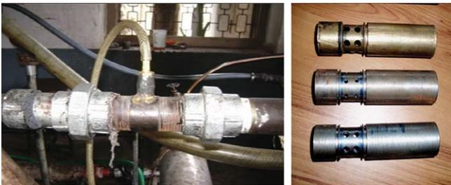
Fig.3: Biogas induction system with mixing venturuses of varied orifice
