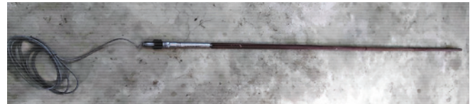
Fig.13: Instrumented rock bolt
