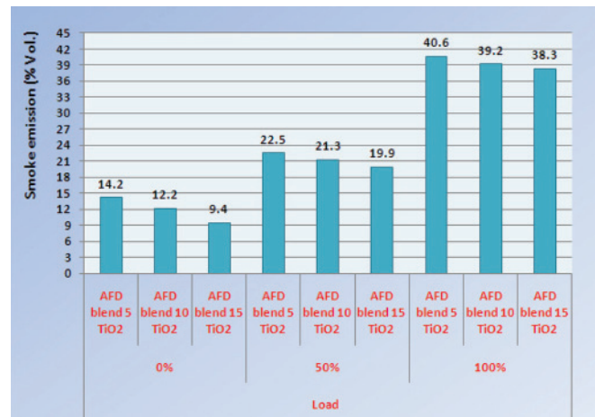
Fig.9 Variation of smoke emission with respect to engine load and AFD - TiO 2 blend
