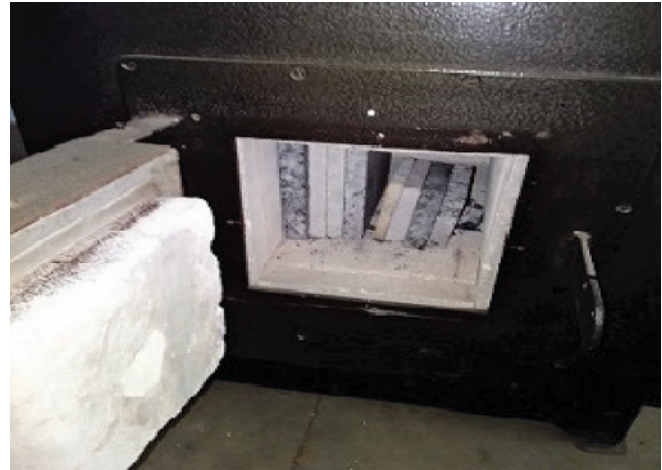
Fig.2: A view of the samples arranged in the heating furnace
