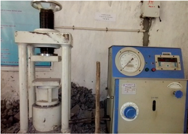
Fig.3: View of the machine used for compressive strength testing of the samples
