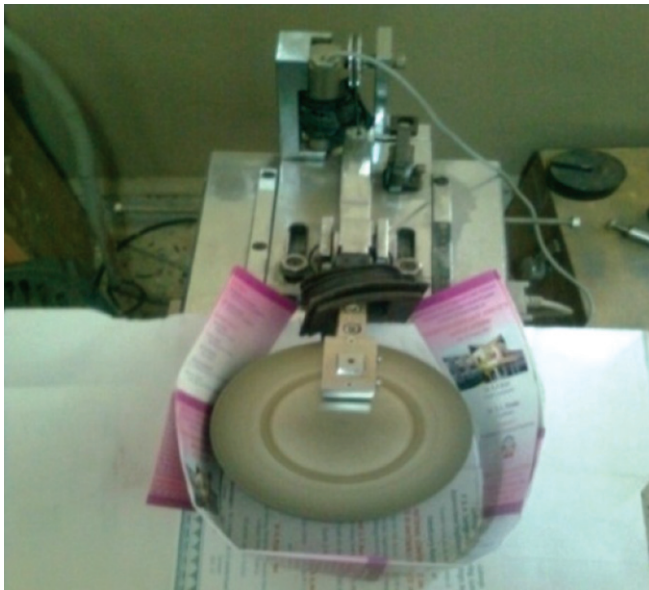
Fig.1: Friction and wear testing machine
