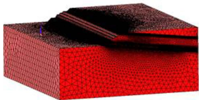
Figure 7. Mesh of the model with opencast mine.
