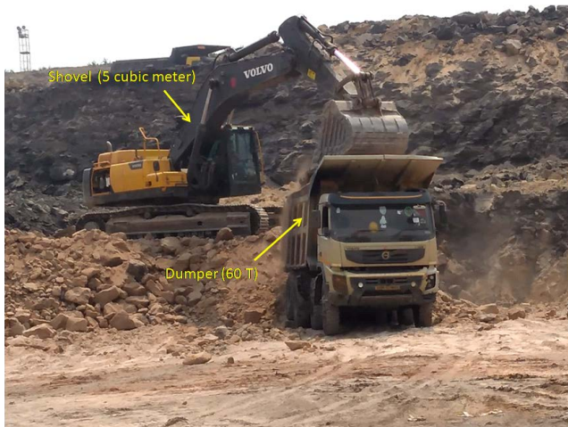
Figure 3. Shovel and dumper working in the mine.
