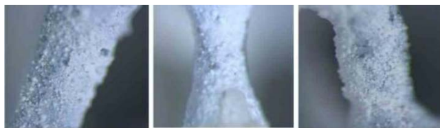
Figure 3. Surface morphology of SiC foam ceramic bars with different dip times.
