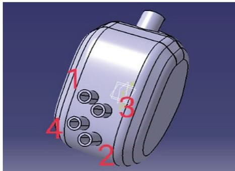
Figure 6: Various Compressed Air Inlet and Outlet
