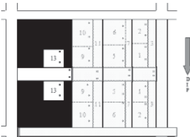
Fig.8: Modified depillaring method of working (full extraction) in conjunction with hydraulic sand stowing, showing 2 faces per SDL per shift (not to scale)
