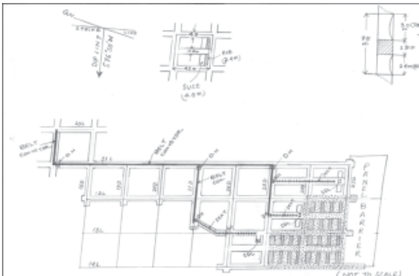
Fig.4: Development with depillaring panel with level splitting in bord and pillar mining
