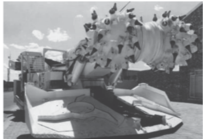
Fig.1 Transverse/ripper type roadheader (Alpine Miner)
