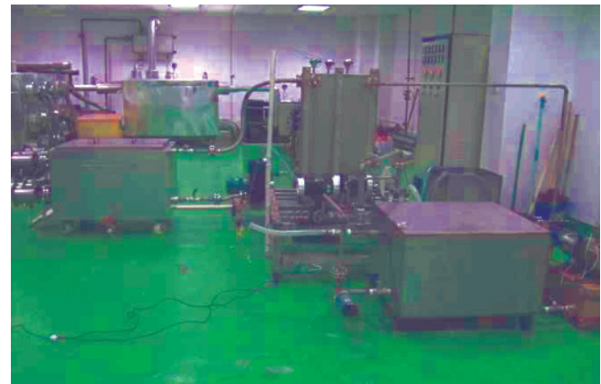
Fig.4 The experiment unit of plate-fin desalination system
