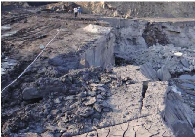
Fig.2 Joint planes perpendicular to highwall slope in T-3 (Bench: 0 to -6 m)
