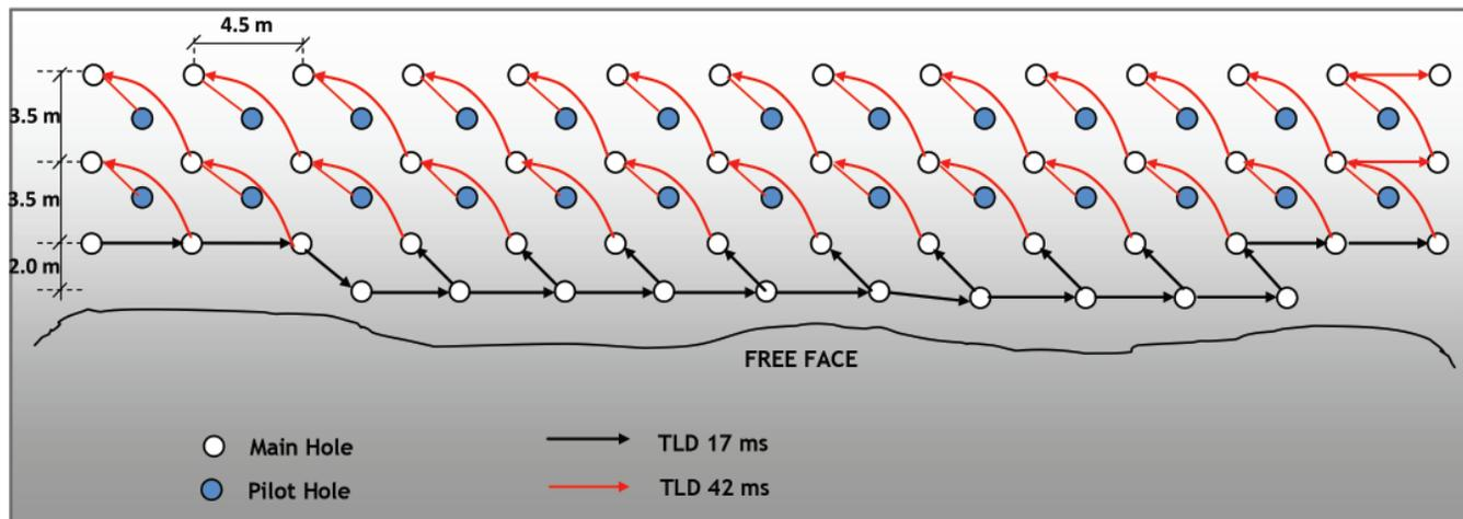
Fig.9 Design pattern of main and pilot/satellite holes for achieving higher powder factor
