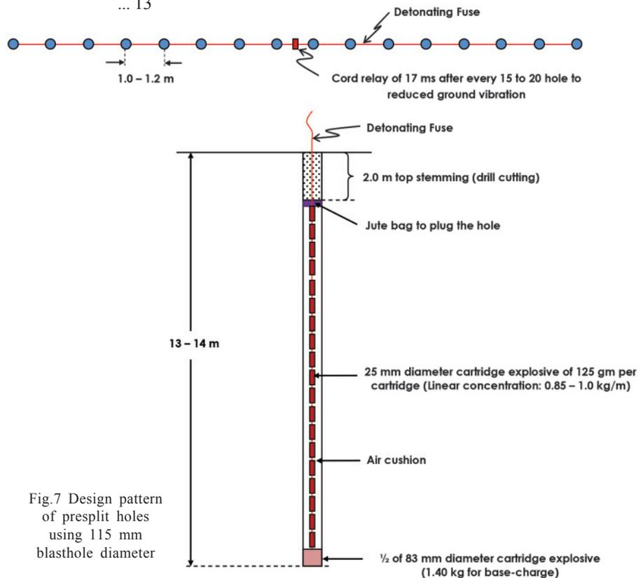
Fig.7 Design pattern of presplit holes using 115 mm blasthole diameter
