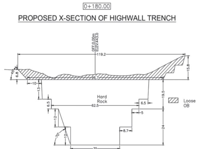
Fig.1 Cross-section of highwall trench at Sharda OCP with 70° slope angle
