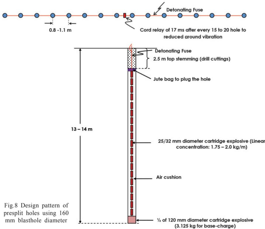
Fig.8 Design pattern of presplit holes using 160 mm blasthole diameter
