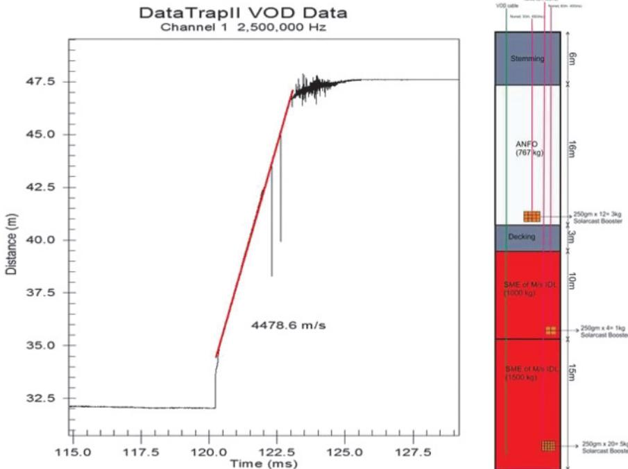
Fig.5 Plot of recorded VOD of ANFO explosive for 311mm diameter blasthole at dragline bench
