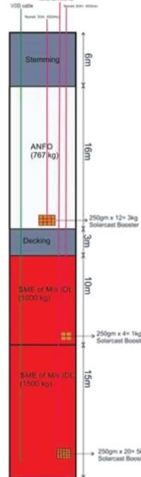
propagation. Stress wave input in blasthole causes simultaneous initiation of explosive throughout column, whereas bottom initiation is followed for real time blast using Nonel or electronic initiation system. The spherical nature of blast wave demands additional booster after certain column length in a long explosive column. Simulated results have been compared to experimental signature hole blast conducted at site.
