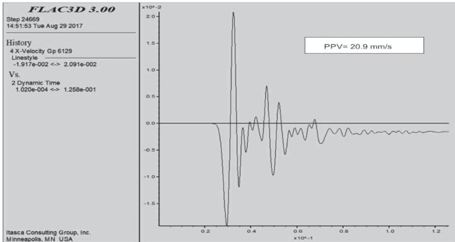
Fig.8 Longitudinal vibration resulted from simulation of blasthole of depth 20m with charge length 14m at radial distance of 50m and longitudinal distance of 43m
