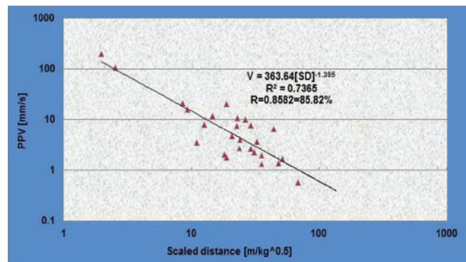
Fig.3 Regression plot of recorded PPV due to blasting at dragline bench faces at their respective scaled distances at Moher and Moher Amlori ext. OCP
