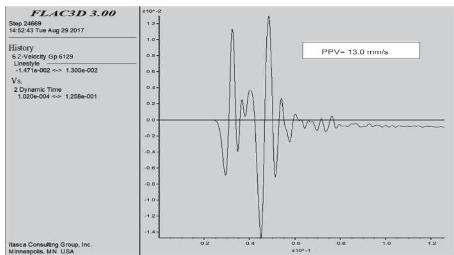
Fig.10 Vertical directional vibration resulted from simulation of blasthole of depth 20m with charge length 14m at radial distance of 50m and vertical distance of 17m
