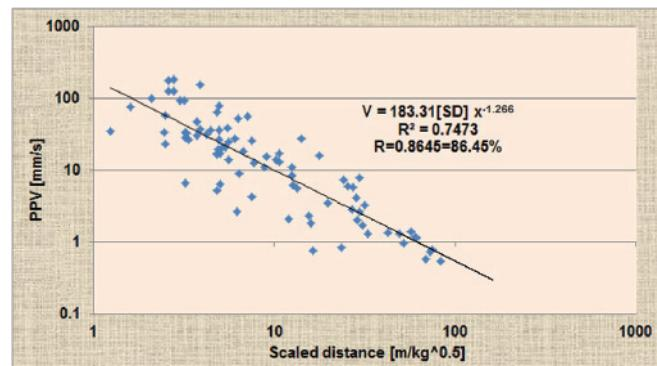
Fig.2 Regression plot of recorded PPV due to blasting at shovel bench faces at their respective scaled distances at Moher and Moher Amlori ext. OCP
