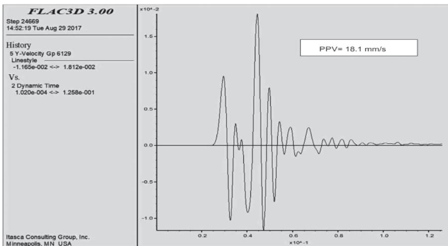
Fig.9 Transverse vibration resulted from simulation of blasthole of depth 20m with charge length 14m at radial distance of 50m and transverse distance of 20m
