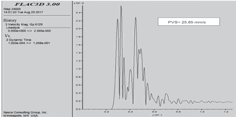
Fig.7 Vibration resulted from simulation of blasthole of depth 20m with charge length 14m at radial distance of 50m, longitudinal distance 43m, transverse distance 20m and vertical distance of 17m
