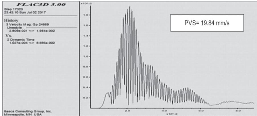
Fig.6 Simulation result of blast vibration recorded at 50m radial distance for blasthole of diameter 100mm and depth 20m with 14m charge column length
