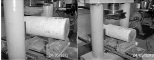
Fig.6 Status of sample before and after applied load
