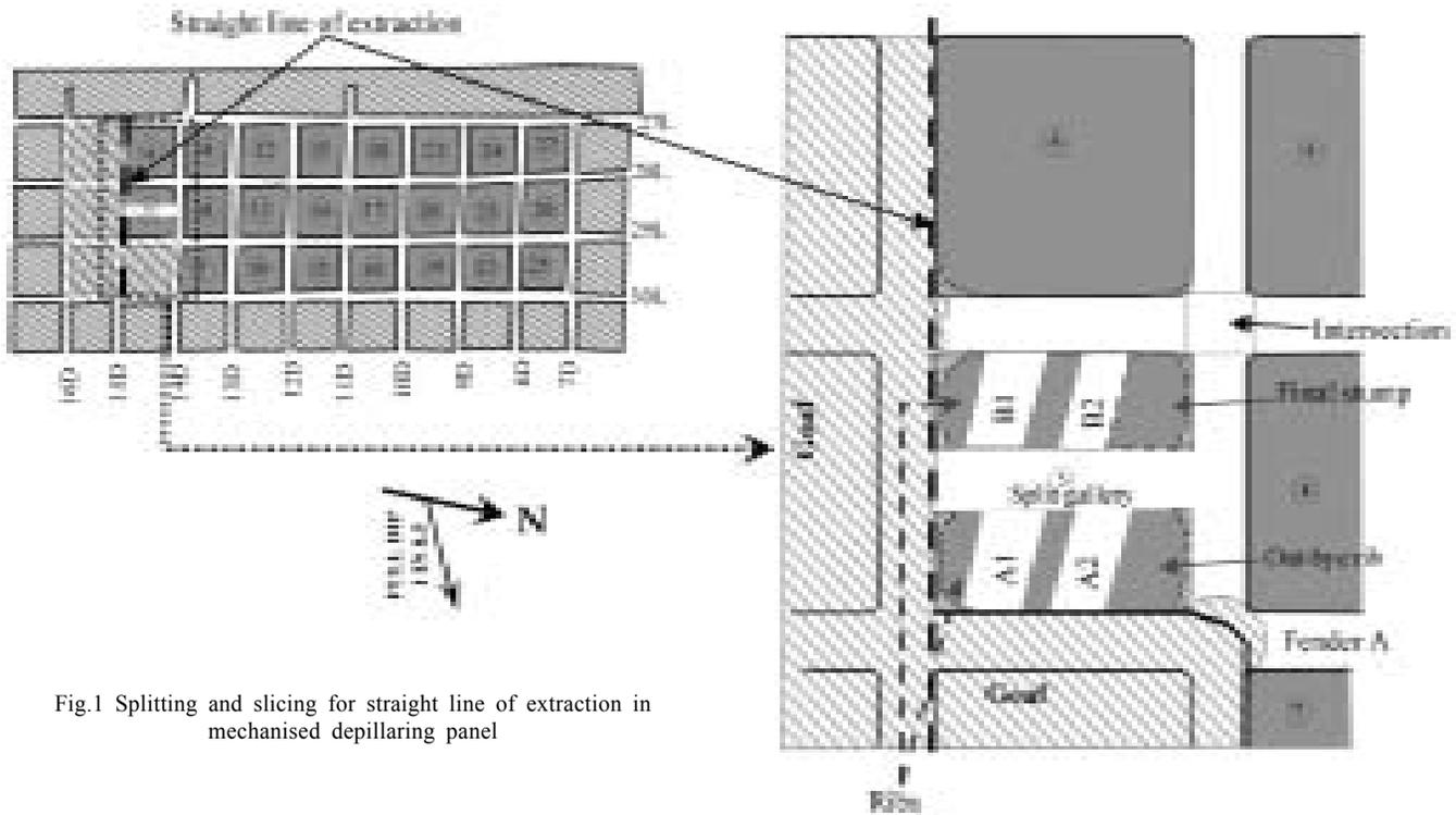
Fig.1 Splitting and slicing for straight line of extraction in mechanised depillaring panel
