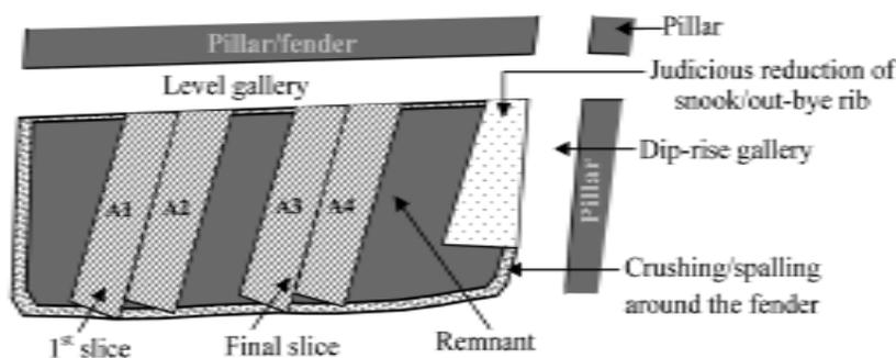
Fig.12 Reduction of a snook through a cut along existing dip rise gallery side in the snook during the mechanized depillaring
