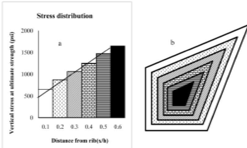
Fig.9 (a) Rib/snook stress distribution (cross-section to the core) and (b) Plan view of the stress distribution in different slices [after Mark and Zelanko, 2001]
