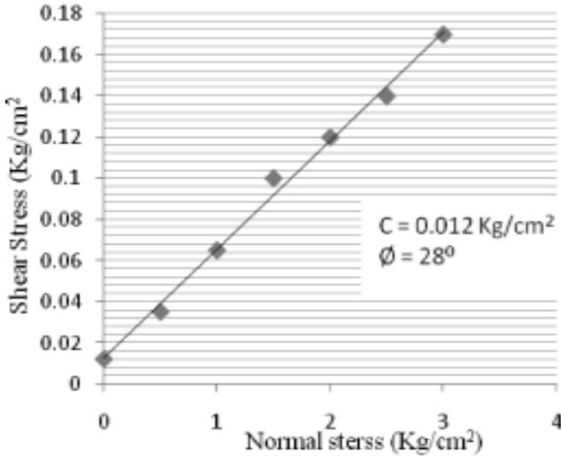
Fig.4 Shear strength test on OB sample
