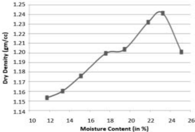
Fig.5 Dry density vs water content of PA
