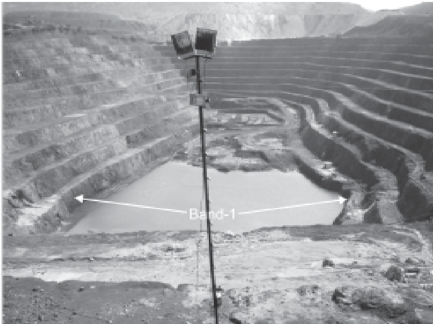
Fig.1 A photograph of open pit mines of M/s Jindal Stainless Steel showing friable chromite Band-I left in barriers between open pit of Tata Steel on the right side and Balasore Ispat on left side. (Courtesy, M/s Jindal Chromite Mine, Kaliapani, Jajpur, Orissa).
