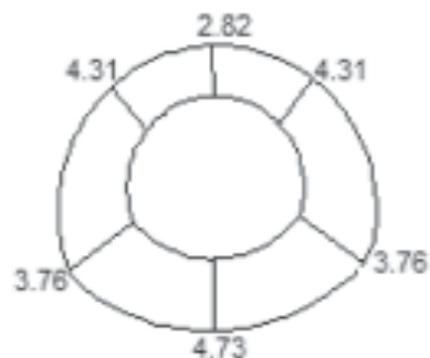
Fig.14 Invert drainage lining safety coefficient
