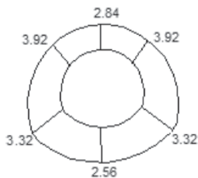
Fig.15 Wall drainage lining coefficient
