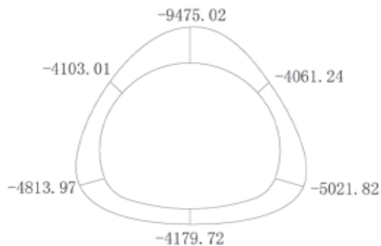
Fig.10 The axial force of invert drainage (unit: kN)
