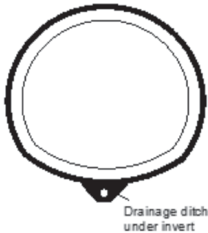
Fig.7 Drainage ditch under invert
