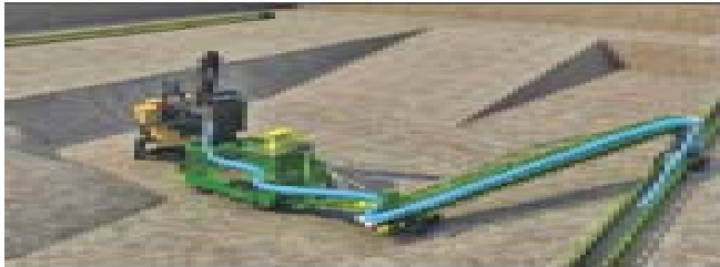
Fig.3 The material conveying flow in semi-continuous technology system
