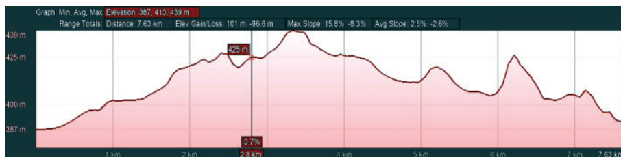
Fig.9 Elevation profile of second pipe conveyor section
