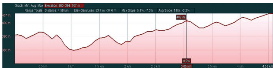
Fig.10 Elevation profile of third pipe conveyor section
