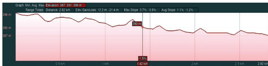
Fig.8 Elevation profile of first pipe conveyor section
