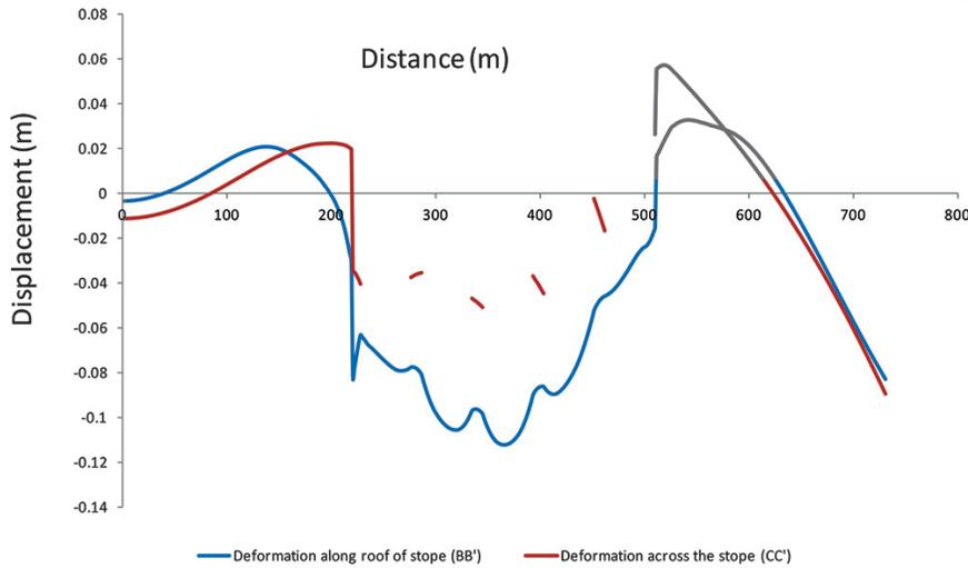
Fig.12 Vertical displacement profile along B-B' and C-C' section
