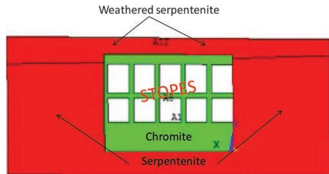
Fig.6 Excavation finite element model
