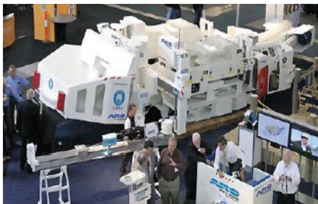
Fig.6 Prototype machine for roof and rib bolting (After Corke P et.al. 2008)
