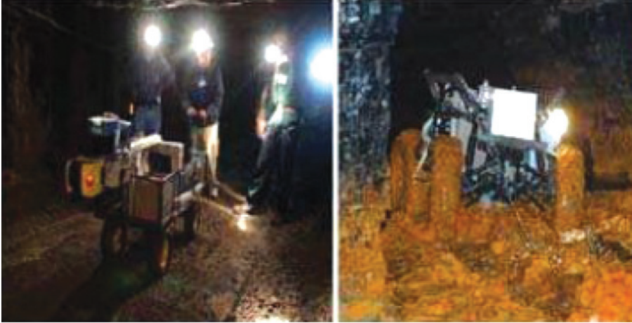
Fig.8 Mine mapping cart with four laser range finders, pushed manually through a mine. Groundhog robot used for breaching difficult mine environment (Courtesy: Nanda S K et.al. 2010)
